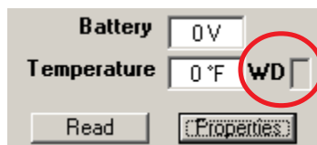
Figure 3-3. Warning Device Indicator
